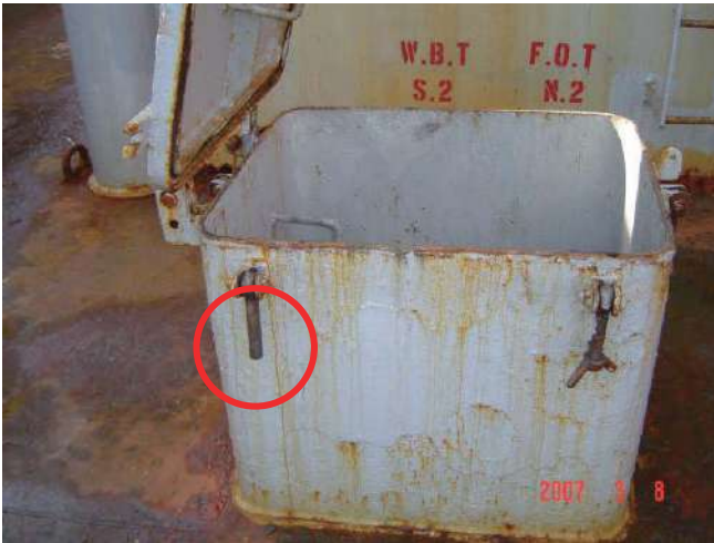
Missing nut of small hatch
