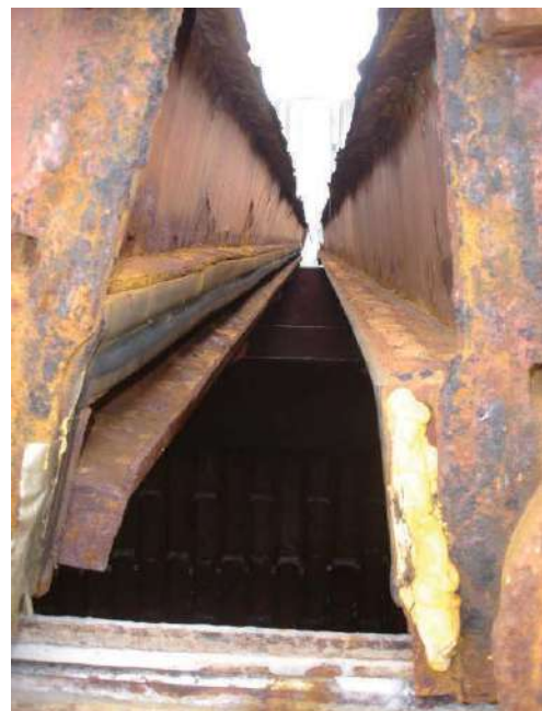
Wastage of cargo hatch covers
