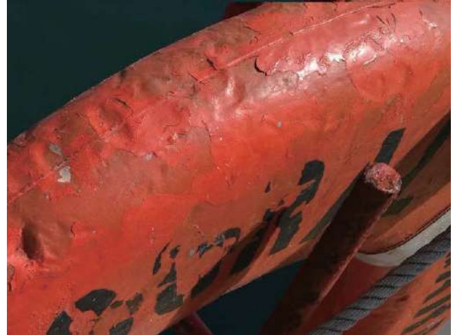
Fading of marking
