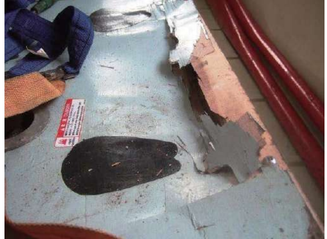
Damaged lifeboat seat
