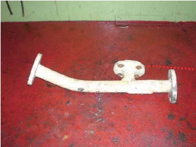
Flange connection to by-pass line
