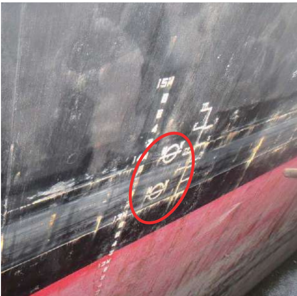
Double marks (Not acceptable)
