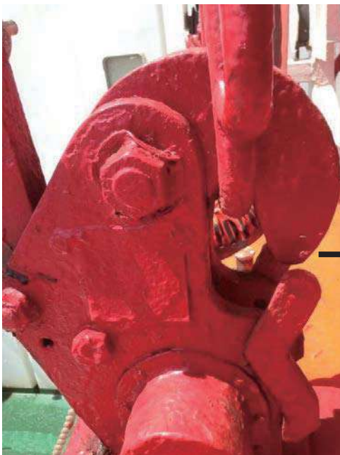
Seize of on-load release gear by excessive paint
