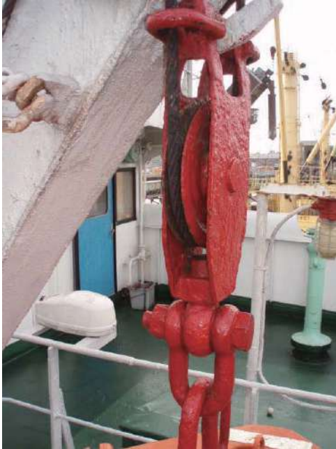
Wastage of boat fall block
