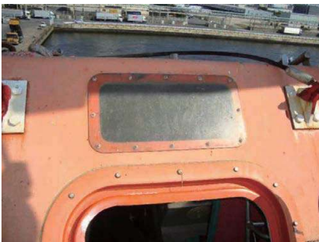
Poor visibility through window
