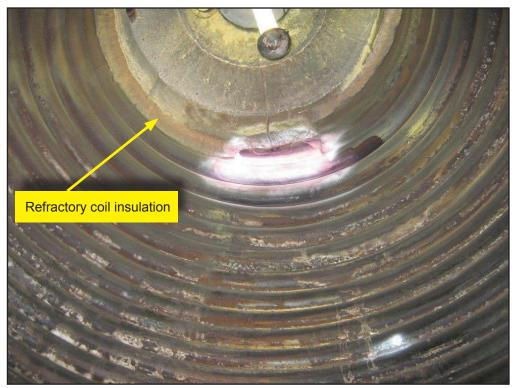
**Figure 7:** Photograph of internal view of a similar thermal oil heater furnace roof showing original refractory
