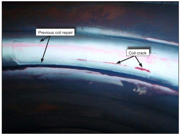
Figure 10: Photograph of port thermal oil heater coil fracture
