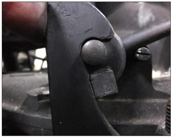
Figure 3b: Photograph showing burner unit latching mechanism (closed)
