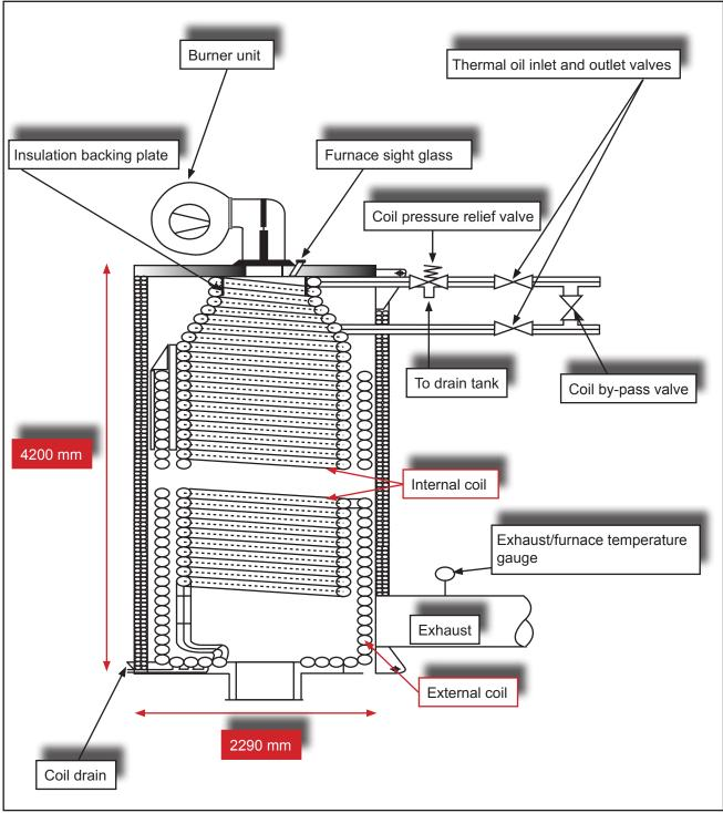
Figure 6: Diagram of the port thermal oil heater
