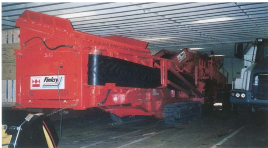
Fig. 14. Tracked vehicle secured on vehicle deck
