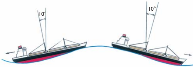
(b) Pitching to 10° bow up and surging astern, and pitching to 10° bow down while surging ahead, as each wave passes.
