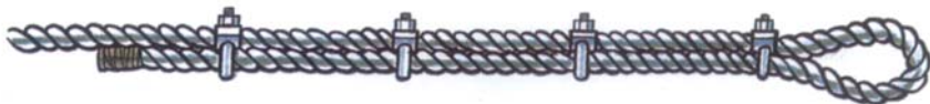
Fig. 4. An eye in a wire rope properly made up using four grips
