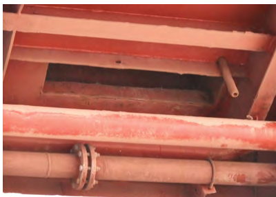
Ventilator opening in deck at the aft bulkhead of cargo hold No. 3. The steel bulkhead is the common boundary between the accommodation and the cargo hold ventilator.
