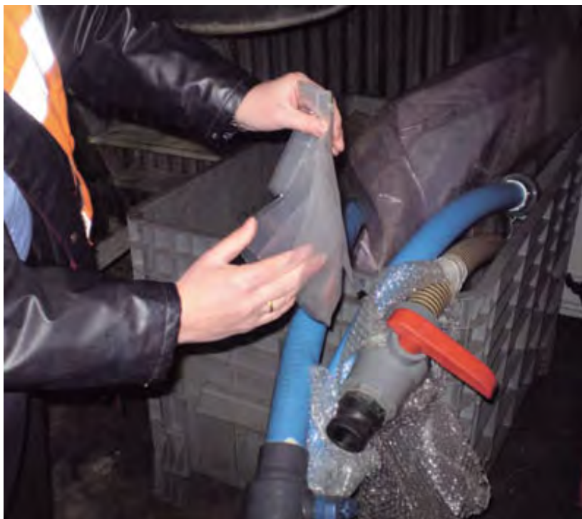
Example of a five-ply plastic flexi-tank.
