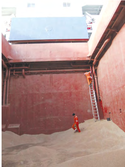
Aft bulkhead of cargo hold No. 3. The ventilator opening is in the corner, above the ladder. Access is difficult, as it is behind pipes under deck.
