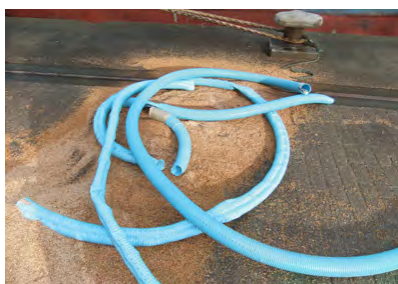
Plastic tubes used for aluminium phosphide tablets, pulled out after discharge of the cargo holds.
