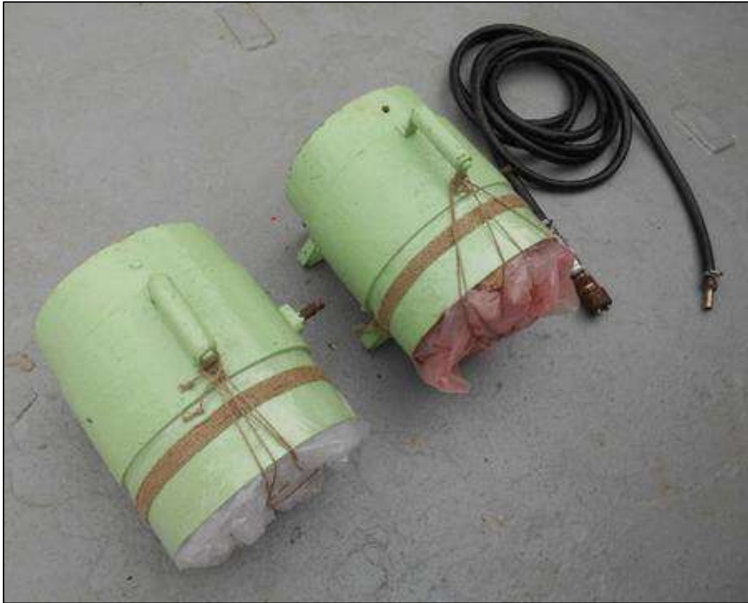
Figure 3: Portable ventilation fans
